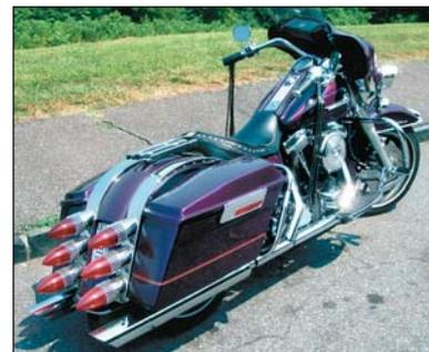
As you can see, the filler strips were chrome plated, and the license plate frenched into the fender, giving the bike a classic lost-in-the-'50s look. The muffler extensions to the Screamin' Eagle exhaust system help balance the look.
