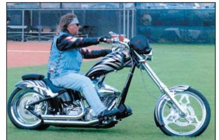
2003 Big Dog Chopper, the first year for what has turned out to be the Kansas-based company's best-selling model. And rightfully so, when you consider the heart of this big dog is a 107-cubic-inch S&S engine linked to a Baker 6-speed overdrive transmission (left-side drive; the RSD wasn't introduced until 2005).
