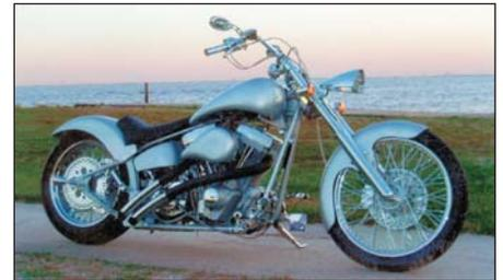
Custom frame that boasts a 36-degree rake and two-inch stretch to the backbone. A stock-length fork with 5-degree raked triple trees and 21" front wheel (18" rear) gives the bike its classic stance. He shoehorned a stock-with-S&S-carb engine into the frame, capping it with Radium exhausts.
